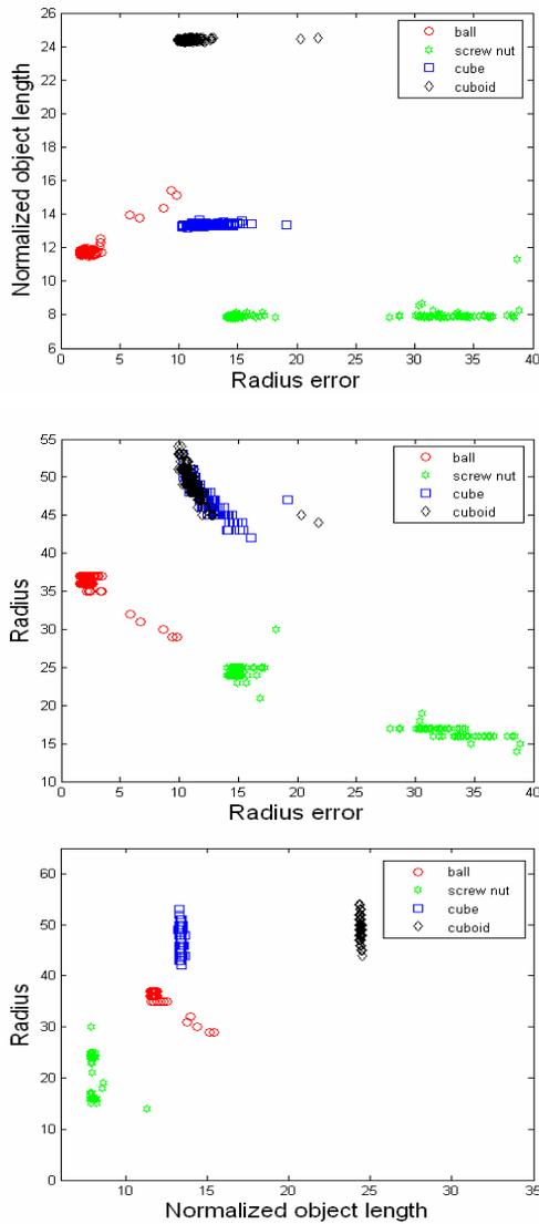
Fig. 10 Illustration of the resulting features distribution in 2D space using the normalized object length vs. the radius error (Top), the radius vs. the radius error (middle) and the radius vs. the normalized object length (bottom)
