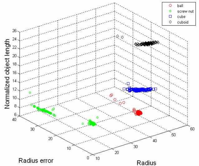
Fig. 9 The resulting features distribution in 3D space from the test-objects using the radius, the radius error and the normalized object length
