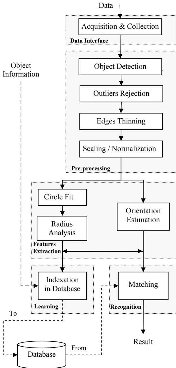
Fig. 3 Overview of the data processing concept
