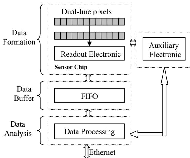
Fig. 1 A system diagram of the smart vision system
