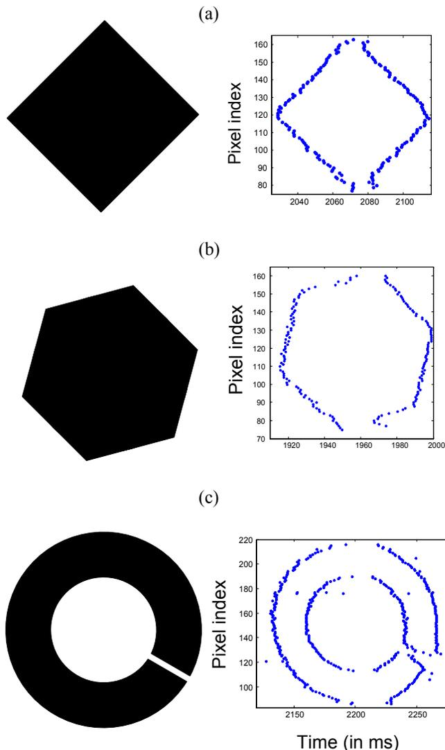
Fig. 2 Original shapes of a quadrangle (a), hexagon (b) and a ring (c) depicted on the left figures. The data representation of those images with the presented vision system are, respectively, given on the right figures
