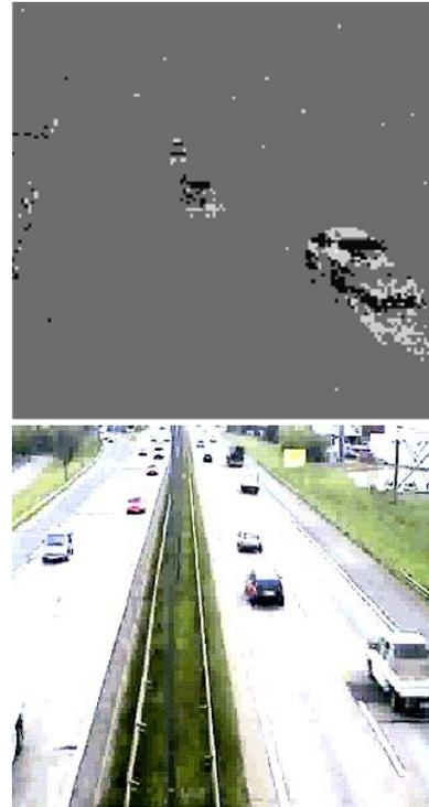
Fig.1 Example of asynchronous AE data represented as a video frame (top) and a video still image of the same scene (bottom).
