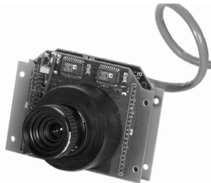
Fig. 3. Photograph of the smart camera system.
