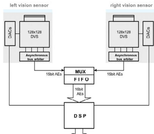
Figure 1: Hardware architecture and signal flow of the Stereo DVS
