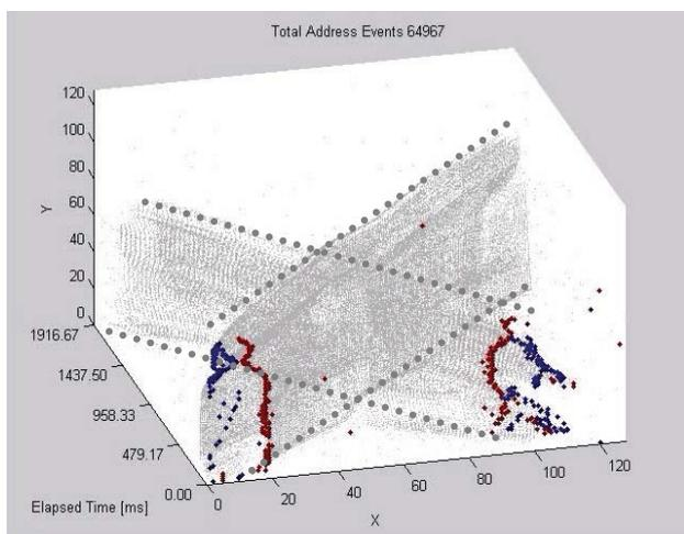
Figure 3: Event representation of scene dynamics (2 persons crossing the field of view) in a space-time domain using 1 DVS
