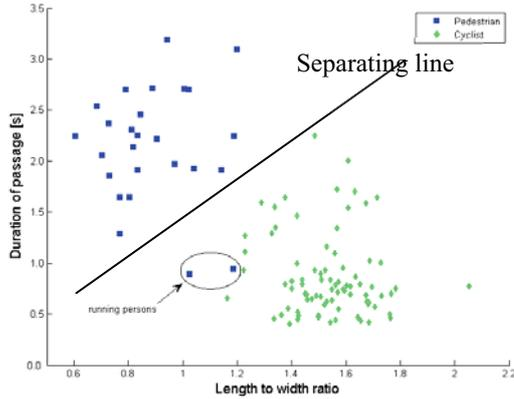
Figure 10: Classification results of riding cyclists and pedestrian using the size vs. passage duration
