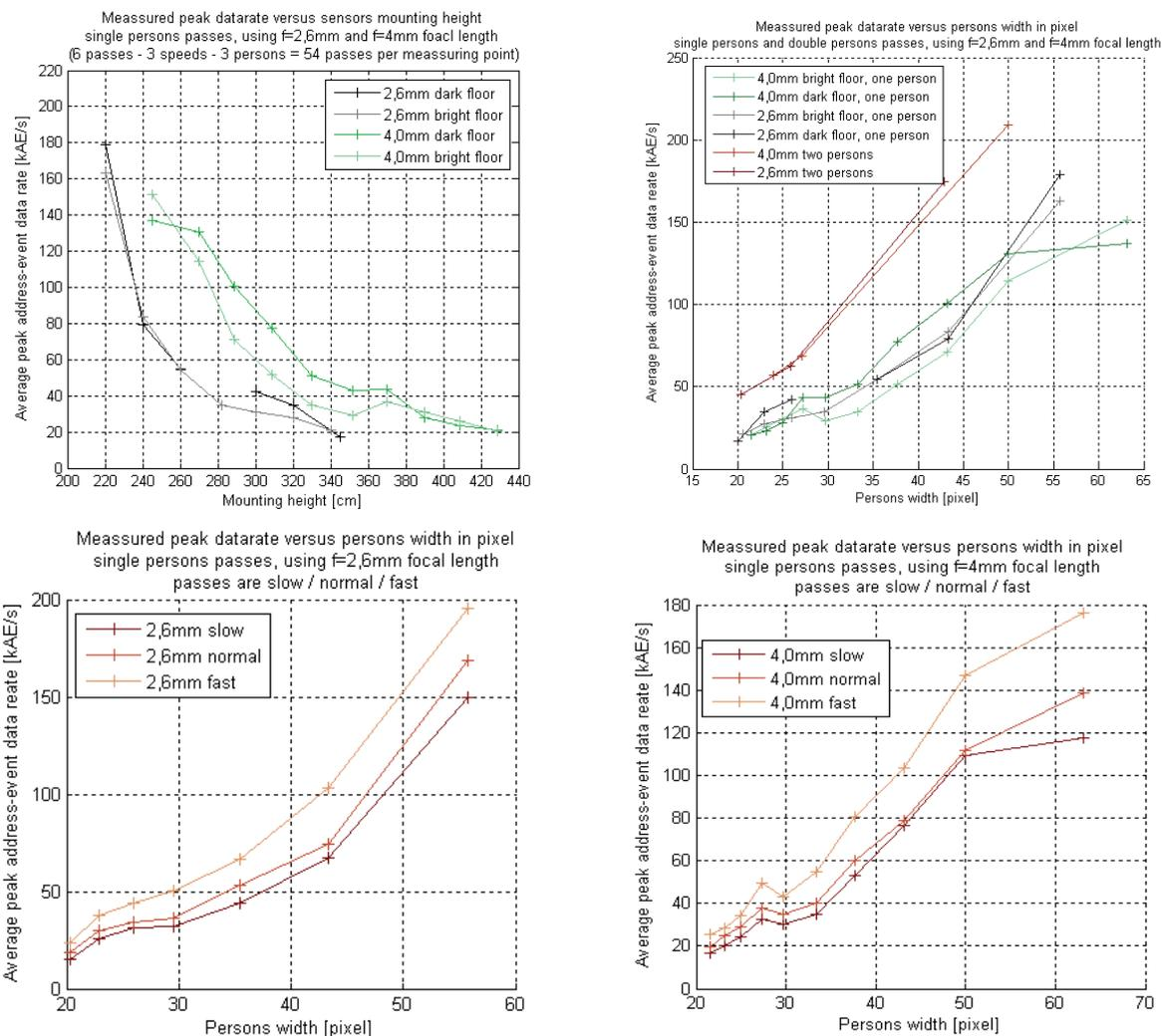
Figure 8: Illustration of resulting data rates for persons crossing the sensor field of view and its dependability on mounting positions & person size
