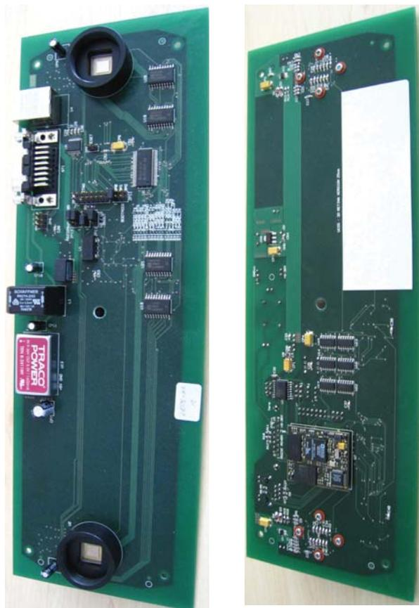
Figure 2: Image of the realized event-based stereo vision system: front face (left) and back face (right)
