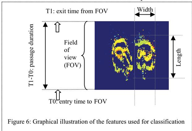
Figure 6: Graphical illustration of the features used for classification
