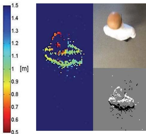
Figure 4: Still image of a person from a conventional video camera (top right); the corresponding AE from one dynamic vision sensors (bottom right); resulting "sparse" event depth map color coded (left)
