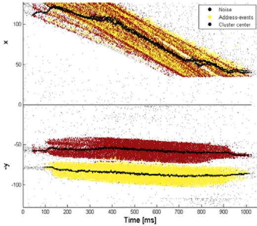
Figure 9: Illustration of tracking two riding cyclists during their passage across the sensor FOV (x-coordinate; y-coordinate; time)
