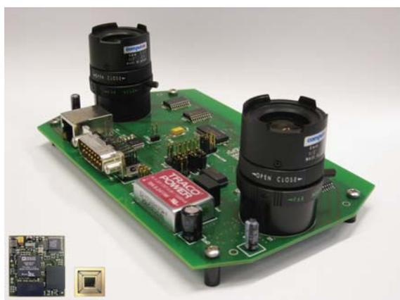
Figure 1: Dynamic stereo vision system device. In the lower left corner the DSP Bf537 and the sensor chip are shown. The DSP is mounted on the back of the board.
